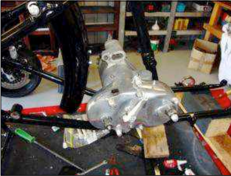
The Ariel gearbox is ordinarily a sturdy piece of equipment but I managed to seize it.
