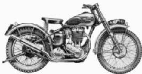
The 1950-53 VCH model weighed 290 lb. and was a popular trials machine. The engine, which developed 25 hp at 6000 rpm, was available with either wide or close ratio gears.
