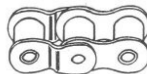
Fig. D8. Double Cranked Link.
