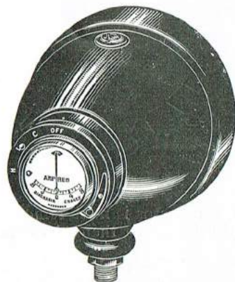
Fig. 4. Head-lamp showing switch complete with ammeter.
